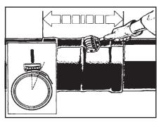
After the DIRAX sleeve has shrunk into the joint area and while it is still hot and soft, run a small hand roller over it to push out any trapped air.
