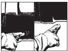
During shrink down, check adhesive flow with finger occasionally. Wrinkles should disappear automatically.
