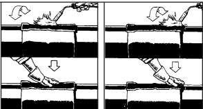
Immediately pat it down firmly with a gloved hand. Continue heating and patting every 10 cm (4") until the whole patch area is finished.
