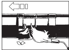
After you have finished heating the side at the leading edge, recover the remainder of the sleeve by heating toward the other end of the sleeve.
