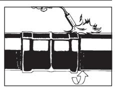
An 80 mm (3.2") wide sacrificial sleeve is installed on the leading edge to function as a wear cone during pull thru of the pipe. Start by heating the leading edge area to 70°C (160°F).
