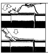
Using a propane torch with a flame length of approximately 500 mm (20"), start heating one end of the closure area.
