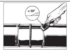
If not factory beveled, chamfer the adjacent pipe coating to an angle of preferably 15°, maximum 30°. Inspect the edge of the existing pipe coating. Disbonded sections have to be trimmed of and the coating edge has to be beveled again. To avoid possible contamination, it is recommended to use a scraper.
