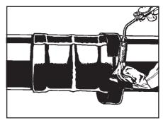
Wrap the leading edge sleeve over the transition DIRAX - mill coating. Make sure that the closure is placed away from the main sleeve closure. Preheat the inside adhesive layer just next to the closure for a few seconds. Press down to make it stick to the other sheet end.
