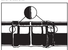
Smooth down the edges of the sleeve with the silicone hand roller.
