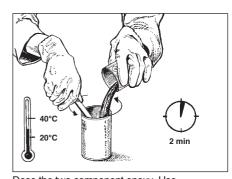
Dose the two component epoxy. Use pre-dosed epoxy kits or use calibrated epoxy pumps.
